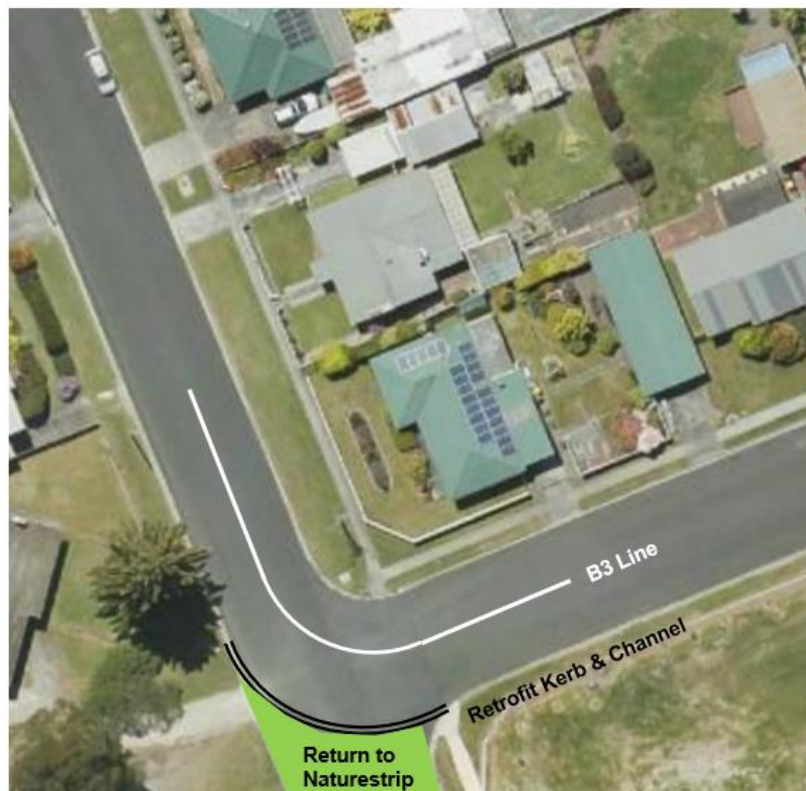
Figure 65.3 – Proposed Austin St / Jenner St corner traffic management.
