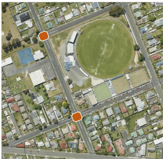
Figure 67 – Proposed Austin Street Traffic Calming with raised plateaus
